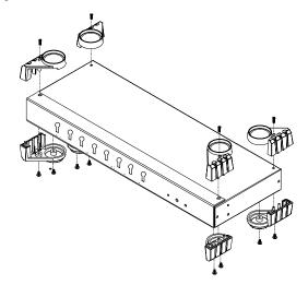
2. Screw the mounting brackets into the sides of the unit, as shown in the diagram below:
